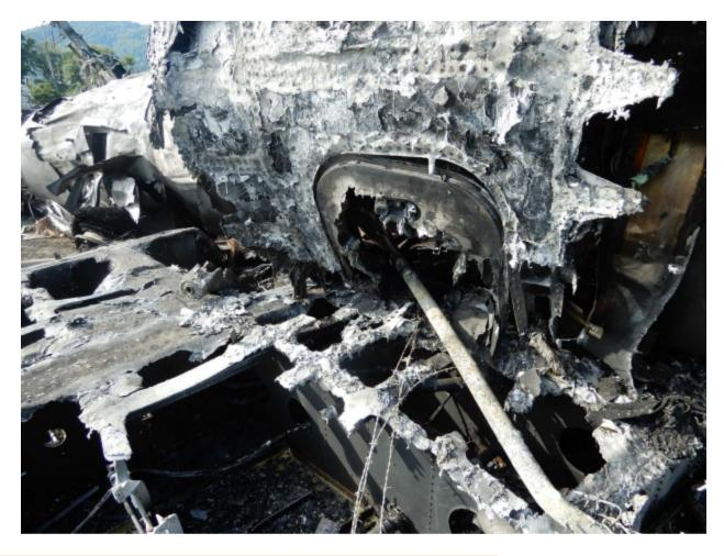
Figure 3: Emergency escape hatch impaled by a metal fence post.
