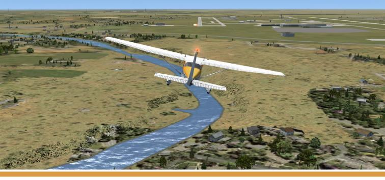
A danger of any kind of slip is getting low. It's critical to keep the angle of attack not only within safe limits but with a margin is it's gusty. And when you're low, there's a tendency to pull the nose up instead of adding power, which can lead to big problems.
