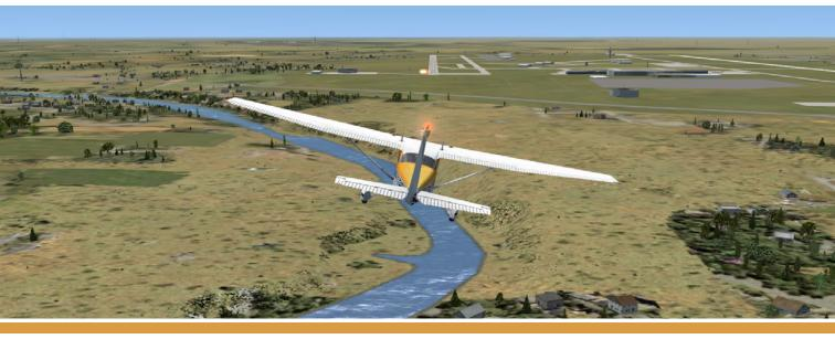
A side slip keeps the nose of the plane pointed where you're headed, or close to it.
